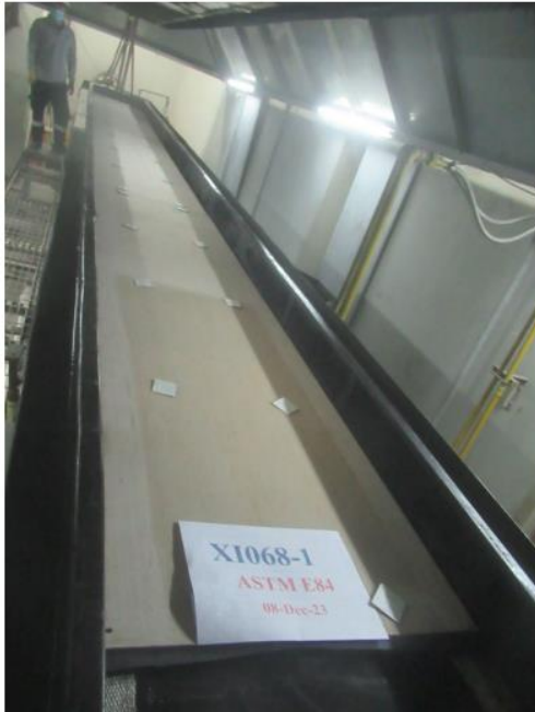
Photo 1: Specimen before the test. (Non-Fire Side)
